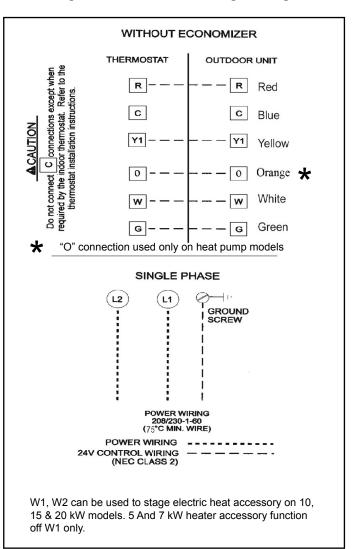
**Figure 4. Typical Wiring Connections**
