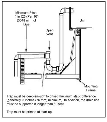
**Figure 5. Typical Condensate Drain Connection**
