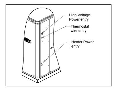
Figure 2. Typical Field Wiring
