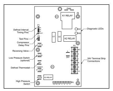
Figure 7. Defrost Control Board
