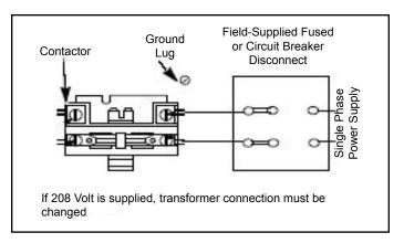
Figure 3. 208/230 Line Voltage Wiring
