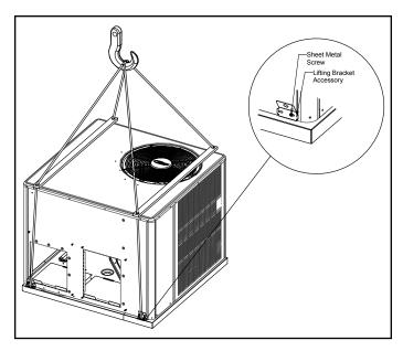
Figure 1. Rigging Unit
