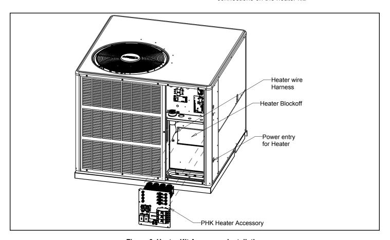
Figure 6. Heater Kit Accessory Installation
